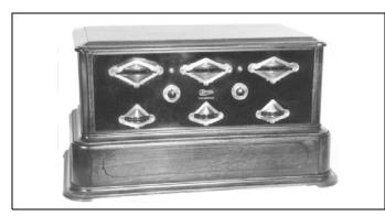
Early to Mid 1930' - "Cathedral". By this time many radios began using the "Superheterodyne" circuit which is the circuit standard to this very day.
